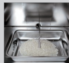
Specimen temperature display with PT 100 sensor
