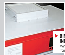
Safety drying oven with HEPA fresh-air filter EU 14
