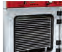
Vacuum drying oven with specific shelves for the placement of large numbers of very flat specimens
